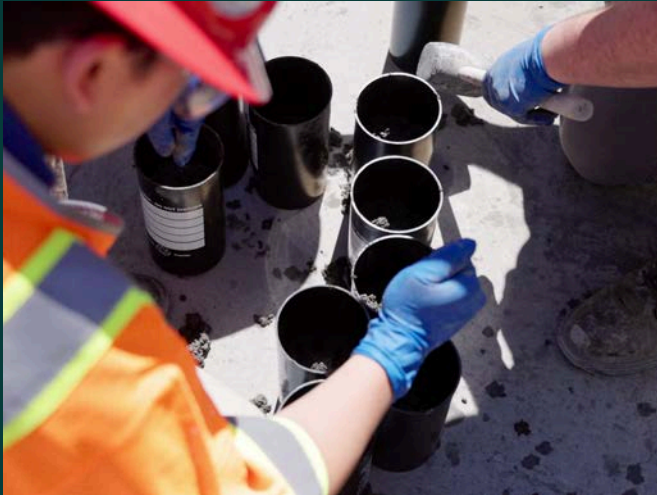
Central Concrete batch testing biochar mix design
